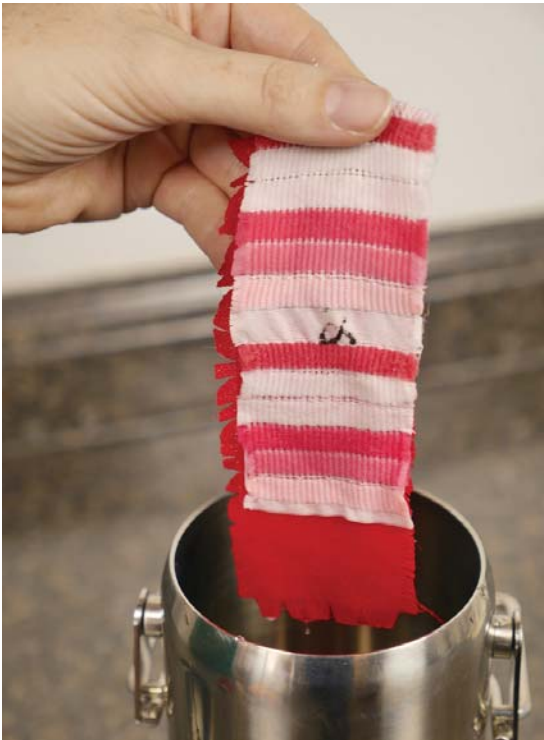
Stained Multifiber from Rotawash Container
